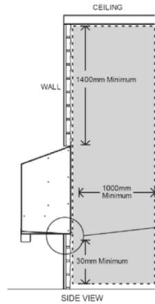
Minimum clearance distance between a combustible ceiling and the fascia must be no less than 1400mm.
