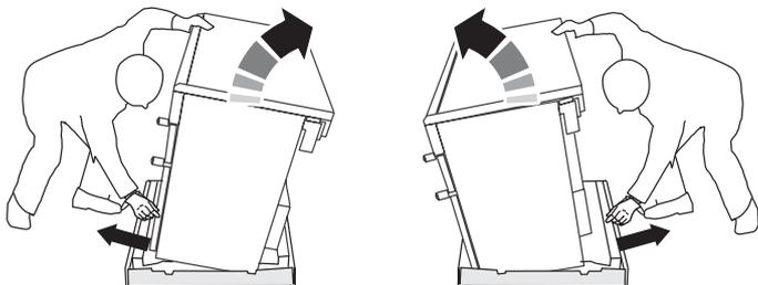
Repeat from the front and remove the front half of the poly base. Pull the drawer out to its furthest point.
