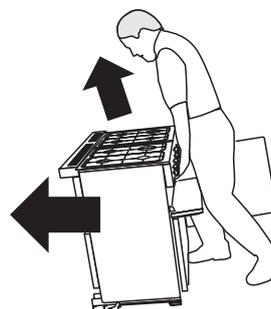
Do not use the door handles or control knobs to manoeuvre the cooker. Use the hotplate and griddle bowl areas.
