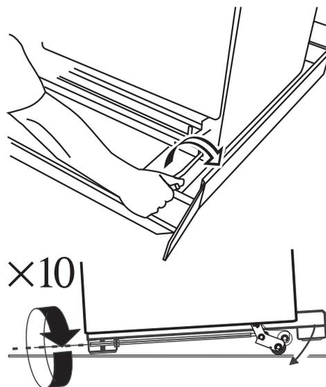
Make sure you lower BOTH REAR ROLLERS. There are two adjusting nuts, one for each roller, at both the front bottom corners of the cooker.
