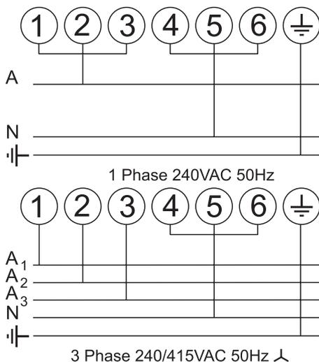
Make sure that the mains characteristics (voltage, nominal power, etc.) match the ratings indicated on the data plate affixed to the lower right hand cooker upright (remove storage drawer). The cooker is preset for a single-phase earthed electrical connection. It is essential to install a multi-pole circuit breaker that completely disconnects the appliance from the mains, with a minimum contact break distance of 3mm.
