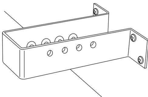
**For both floor and wall attachment it is essential to use the appropriate fixing screws and to ensure that the Anti-Tip Bracket is firmly attached .**
