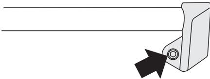
Pull off the push fit control panel end caps at each end and remove the end fixing screws under the end cap.
