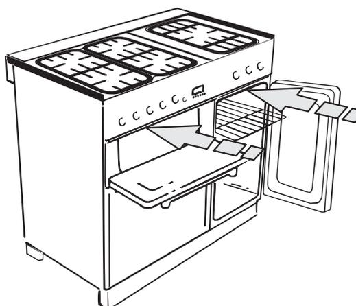
Carefully push the cooker backwards off the pack base. Remove the pack base tray. Position the cooker close to its final position leaving just enough space to get behind it.
