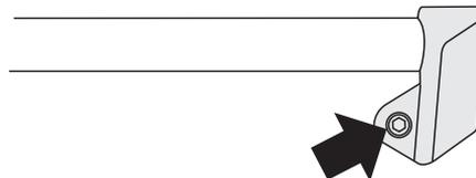
Pull off the push fit control panel end caps at each end and remove the end fixing screws under the end cap.
