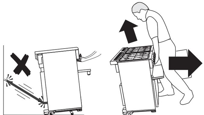
*If a stability chain is fitted, release it as you ease the cooker out. Don't forget to refit it when you replace the cooker.*
