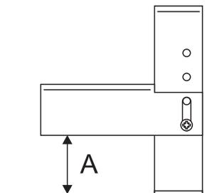
Dimension 'A' should be set to give a clearance of about 6 mm above the center channel of the cooker base.
