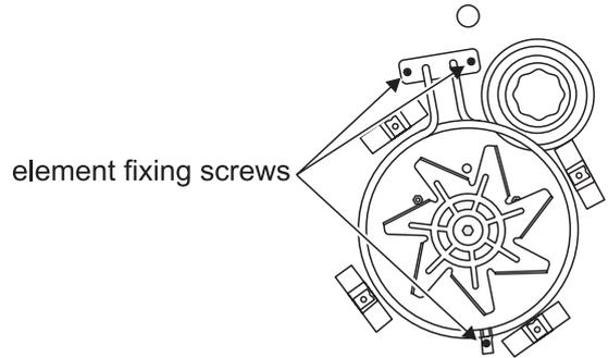
Remove 2 screws from the top of the element and 1 from the bottom of the element in side the oven. Lift element out carefully, disconnect the terminals connected to the element noting their positions. If it is not possible to disconnect the leads in this way, pull cooker forward to gain access to the rear, remove screws securing the electric cover to the back sheet and remove cover and disconnect the terminals from the rear.
