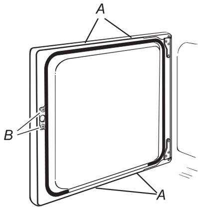
Carefully lift off the outer door panel.
