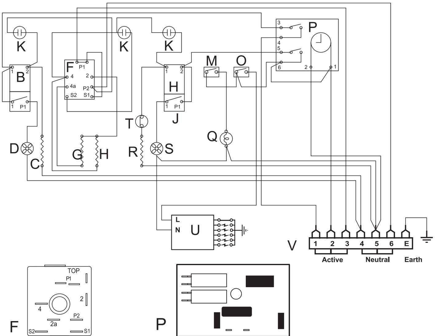
Connection shown in circuit diagram is for single phase.
