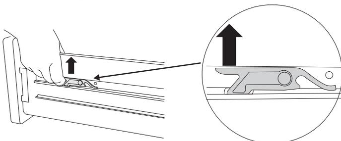
Lift up the ends of the plastic clips (one each side) to release the catches holding the drawer to the side runners and at the same time pull the drawer forward and away from the side runners. For safety's sake push the drawer runners back out of the way.
