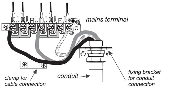
Fix conduit to conduit mounting bracket on the back panel. Connect mains cable to correct terminals for your electrical supply type. Check that the links are correctly fitted and the terminal screws are tight. Replace electric terminal cover box making sure that the conduit is clear of the bottom flange.
