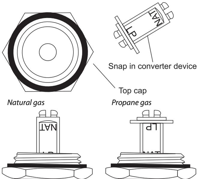
The snap in converter device is marked to show which gas it is set for. Make sure the device is secure in the top cap and refit the cap to the gas pressure regulator.
