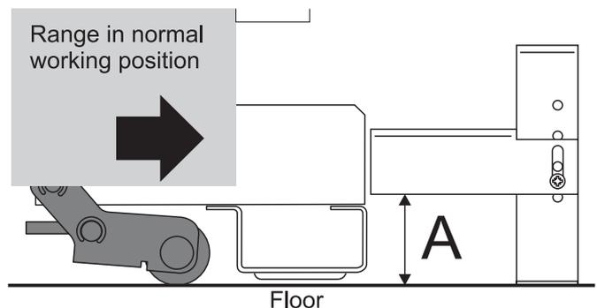
The assembled bracket should be firmly secured to the floor to give a minimum engagement of 50 mm in the center channel of the cooker base.
