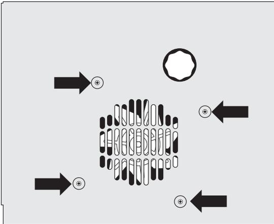
Carefully lift away the inner back. Reassemble in reverse order making sure that the 4 screws and washers are fully tightened.
