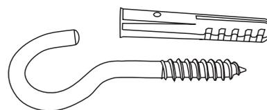
Fix the supplied hook securely to the fabric of the building. Measure the length of chain required. Use the clamp supplied to clamp onto the gas pipe as shown.
