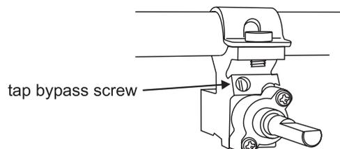
Remove the tap bypass screw and fit the correct new one. See table for correct screws.
