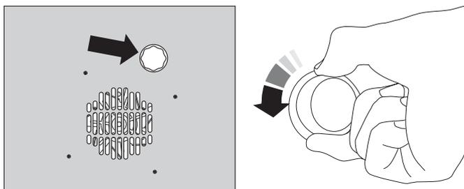
Taking care to protect your fingers in case the bulb should shatter, unscrew the old bulb.
